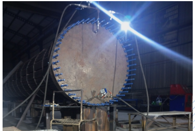
Hydro testing of heat exchanger
